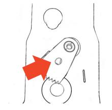
Line up the side of the sector gear, with the notch on the turbine side of the CHRA. Keep in place, do not move.
